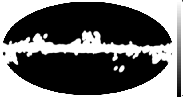
Fig. 2. Mask used for the specific processing of the Galactic center. Precisely, the IRIS map is used as an extra observation in the Galactic part of the mask. The sky coverage is about f_{sky} = 82\% .
